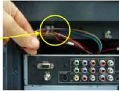
1. Take out the Speaker Right Wire from Wire Clip
