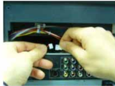
2. Disconnect the Speaker Right Wire
